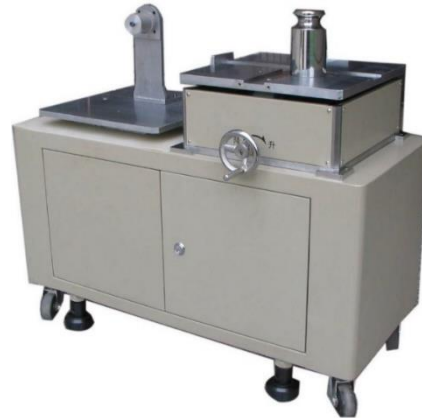
Mass and center of gravity of inertia tester for satellite momentum wheel
